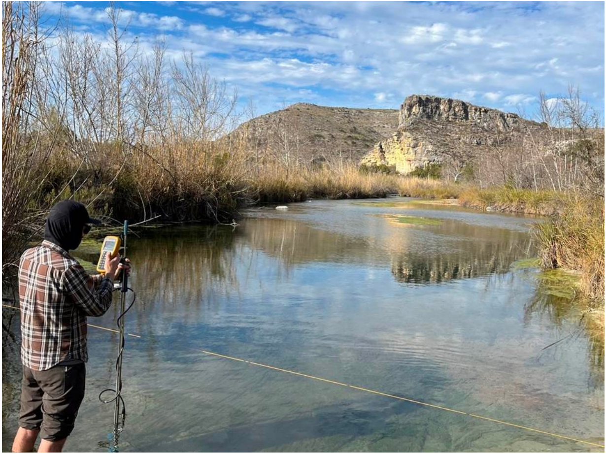
Streamflow measurement taken by Tyson McKinney at Dolan Creek, a spring-fed tributary of the Devils River, Val Verde County. Photo by Brian Hunt.
